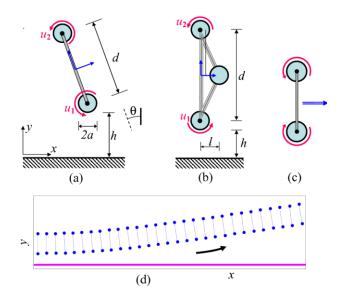
**Fig. 1.** (a) The two-sphere swimmer. (b) The 2+1-sphere swimmer. (c) The two-sphere swimmer with  $u_1 = -u_2$  in unbounded fluid. (d) Snapshots of the two-sphere swimmer with  $u_1 = -u_2$  near a wall
