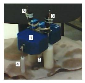
**Fig. 5.** Picture of swimmer with 2+1-cylinders 1. Foam Flotation 2. Nylon Cylinders (2.54cm diameter) 3. Motors / Tracking Markers 4. Nylon Cylinder (1cm diameter)
