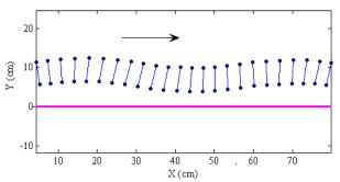
**Fig. 7.** Motion measurements of the 2-cylinder swimmer periodic motion near the wall with unequal motor voltages (wall is at y=0).
