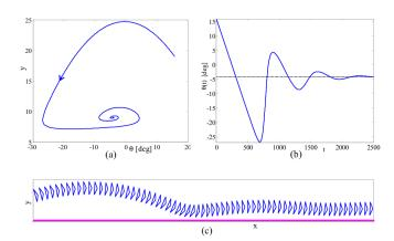
**Fig. 3.** (a) Phase portrait in  $(y,\theta)$ -plane for the 2+1-sphere swimmer near a wall under constant input. (b) Time plot of  $\theta(t)$ . (c) Snapshots of the swimmer's motion
