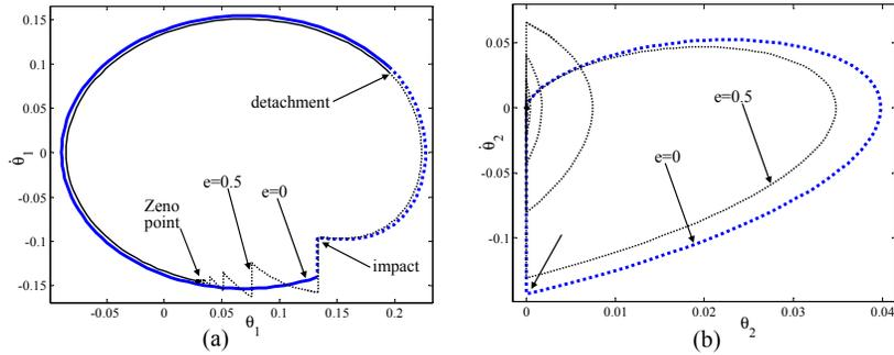
**Fig. 5.** Phase portraits of the periodic orbit in (a)  $(\theta_1, \dot{\theta}_1)$ -plane and (b)  $(\theta_2, \dot{\theta}_2)$ - plane for  $e = 0$  (thin black) and  $e = 0.5$  (thick blue)
