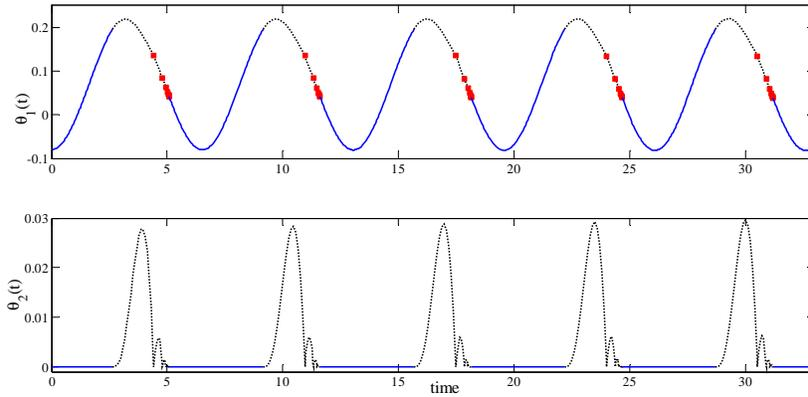
**Fig. 4.** Time plots of the solution  $\theta_1(t)$  and  $\theta_2(t)$  of the controlled double pendulum with  $e = 0.5$ .
