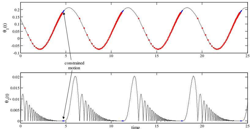
**Fig. 6.** Time plots of the solution  $\theta_1(t)$  and  $\theta_2(t)$  of the controlled double pendulum with  $e = 0.9225$ .
