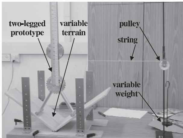
Fig. 5. Experimental setup of a two-legged prototype.
