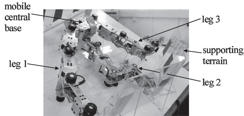
Fig. 1. A three-legged robot moving in a two-dimensional gravitational environment (the mechanism is supported by frictionless air bearings against the inclined plane).
