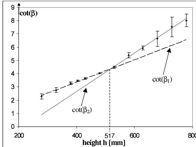
Fig. 7. Experimental (dots) and theoretical (solid and dashed lines) results of  $\cot(\beta)$  as a function of  $h$ . The bars represent two standard deviations.
