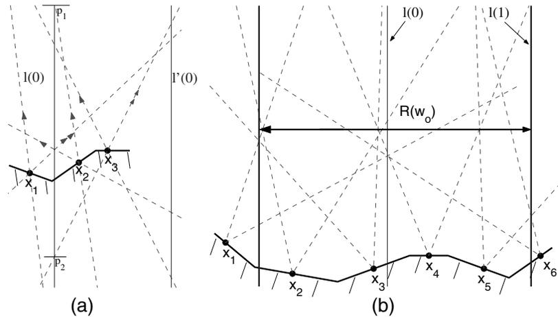
Fig. 8. (a) Illustration of the separation condition (right-pointing lines are double arrowed). (b) Execution of the algorithm on a 6-contact stance.
