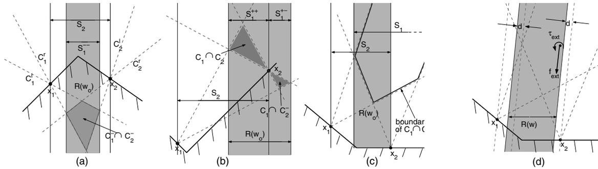
Fig. 3. Graphical characterization of  $\mathcal{R}(\mathbf{w})$  in four cases: (a)  $\mathcal{R}(\mathbf{w}_0) = S^- \cap \Pi$ , (b)  $\mathcal{R}(\mathbf{w}_0) = S^{++} \cup S^{+-}$ , (c)  $\mathcal{R}(\mathbf{w}_0) = S_1^{++} \cap \Pi$ , (d)  $\mathcal{R}(\mathbf{w})$  for a general wrench  $\mathbf{w} = (f_{ext}, \tau_{ext})$ .
