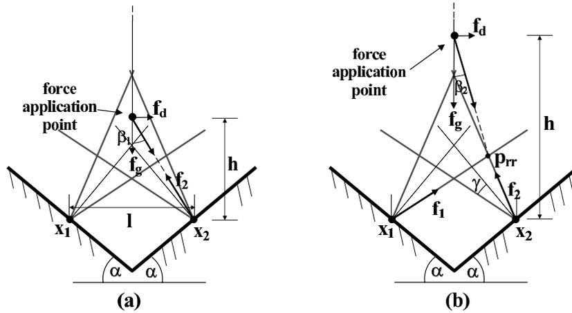
Fig. 6. Graphical characterization of critical disturbance force: (a)  $\|f_d\| = mg \tan(\beta_1)$ , and (b)  $\|f_d\| = mg \tan(\beta_2)$ .
