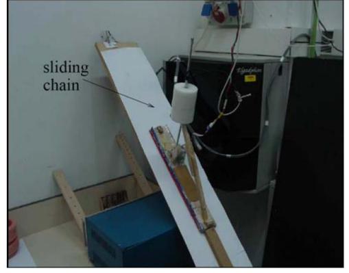
Fig. 4 A prototype of the IPOS mechanism sliding on an inclined plane under the influence of gravity.
