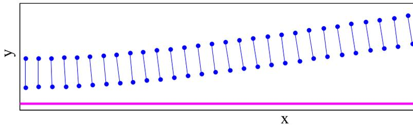
FIG. 2: Snapshots of the motion of the two-sphere swimmer near a wall for  $u_1 = -u_2$
