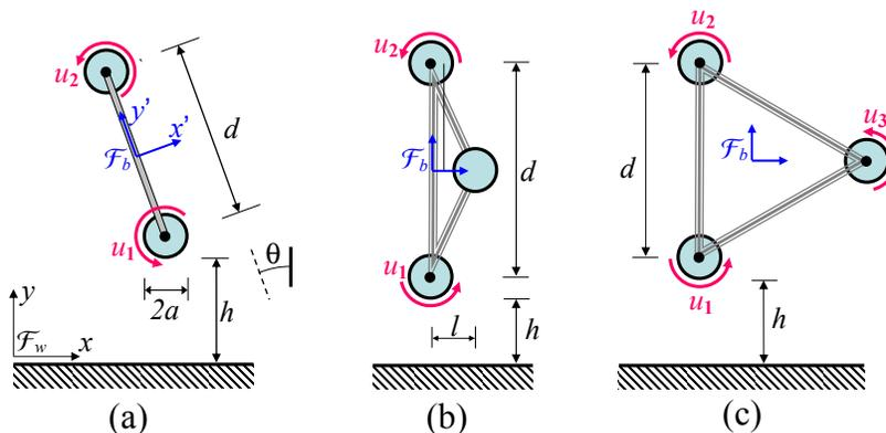
FIG. 1: Drawing of the swimmers. (a) Two-sphere swimmer. (b) 2+1- sphere swimmer. (c) Three-sphere swimmer.
