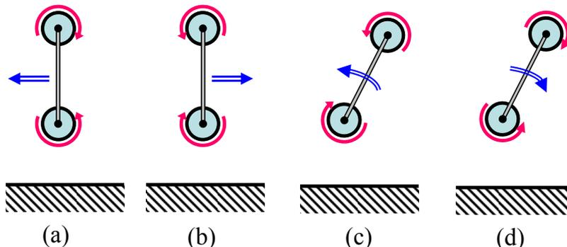
FIG. 3: The two-sphere swimmer near wall - Illustrative explanation of the inherent impossibility of asymptotic stability at  $\theta = 0$ .
